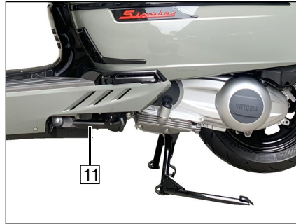
7. Side (11) switch at horizontal position.
