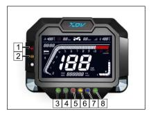
Turn on the scooter every time, the scooter will initialize automatically:self-inspection and all signal lights on, the pointer swings and turn to zero. If the pointer didn't move, please go to dealer to check.
