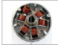
Correct assembly: from the inside out, all the rollers are placed in the position shown in the picture. The exposed iron surface is on the right side and the plastic wrap surface is on the left side.
