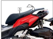
1. Turn ignition switch to "SEAT FUEL" (1), press button "SEAT"(2), open the seat cushion (3).
