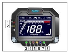
Turn on the scooter every time, the scooter will initialize automatically:self-inspection and all signal lights on, the pointer swings and turn to zero. If the pointer didn't move, please go to dealer to check.
