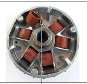
Correct assembly: from the inside out, all the rollers are placed in the position shown in the picture. The exposed iron surface is on the right side and the plastic wrap surface is on the left side.
