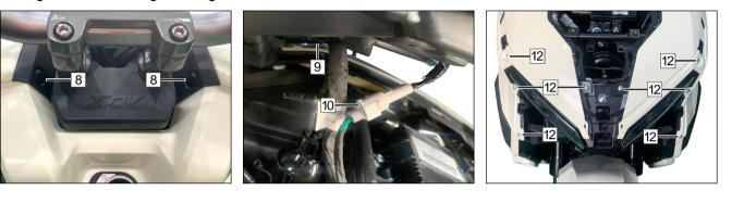
Remove screws (6)(7)(8), unplug connectors (9) (10), windshield bracket, and front panel (11).
