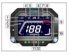
1. Engine coolant temperature indicator Shows the engine water temperature value in real-time.
