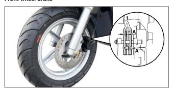
Checking the brake linings
