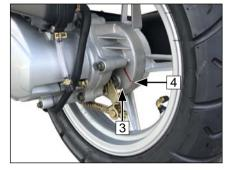
Adjusting the rear wheel brake
