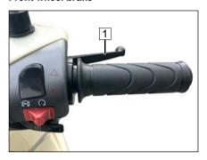
Sudden changes in play or a spongy feel WARNING of the brake lever (1) can be caused by faults in the hydraulic system.
