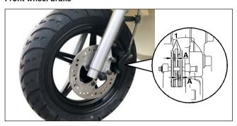
Checking the brake linings
