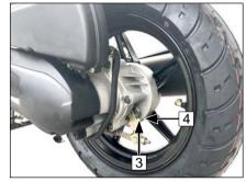
Adjusting the rear wheel brake
