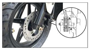
Checking the brake linings
