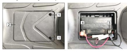
CAUTION The battery may only be connected or disconnected while the ignition is inactive.
