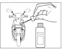
Minor paint damage should be immediately repaired.
