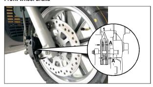
Checking the brake linings
