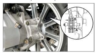
Checking the brake linings
