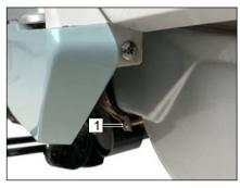
Disassembly and Cleaning the sponge remove the screw(1) and take off the air cleaner, cover L.
