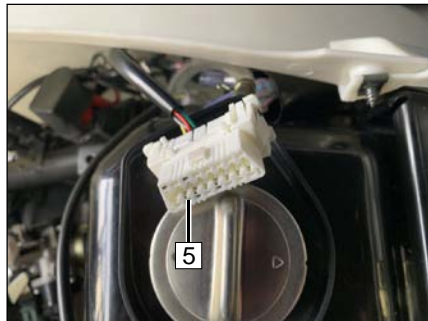
3. Fault diagnosis tester connector (5).
