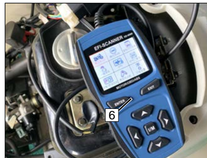
4. Fault diagnosis tester (6).
