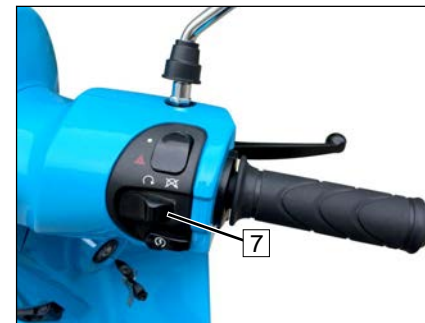
5. Right switch(7) at "↻" position.
