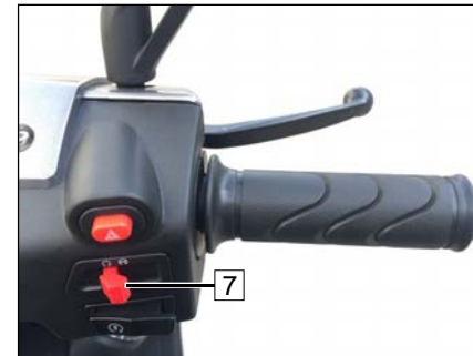
5. Right switch(7) at "ON" position.
