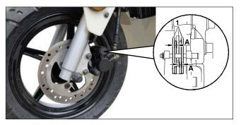
Checking the brake linings
