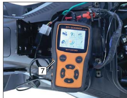
4. Fault diagnosis tester (7).
