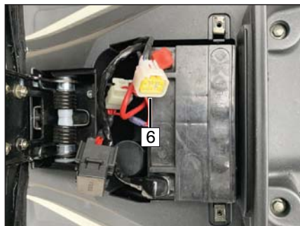
3. Fault diagnosis tester connector (6).
