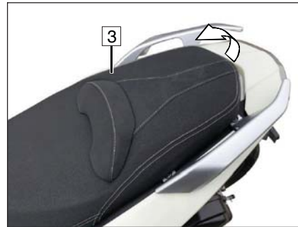
1. Turn ignition switch to "SEAT FUEL" (1), press button "SEAT"(2), open the luggage box (3).
