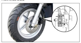
Checking the brake linings
