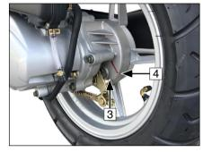
Adjusting the rear wheel brake
