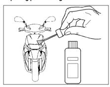
Minor paint damage should be immediately repaired.
