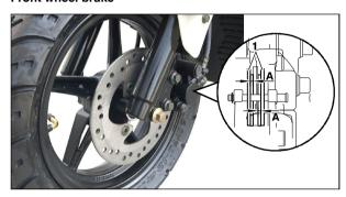
Checking the brake linings
