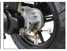
Adjusting the rear wheel brake
