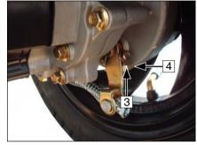
Adjusting the rear wheel brake
