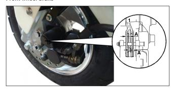
Checking the brake linings
