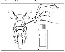
Minor paint damage should be immediately repaired.
