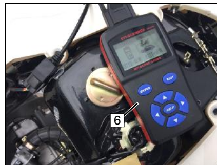
4. Fault diagnosis tester (6).
