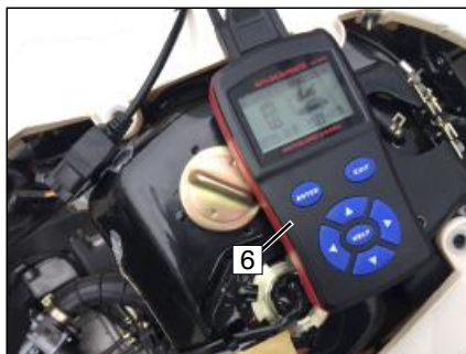
4. Fault diagnosis tester (6).
